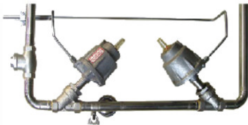
Pipeline system adopts stainless steel sanitary pipe and world brand pneumatic valve
